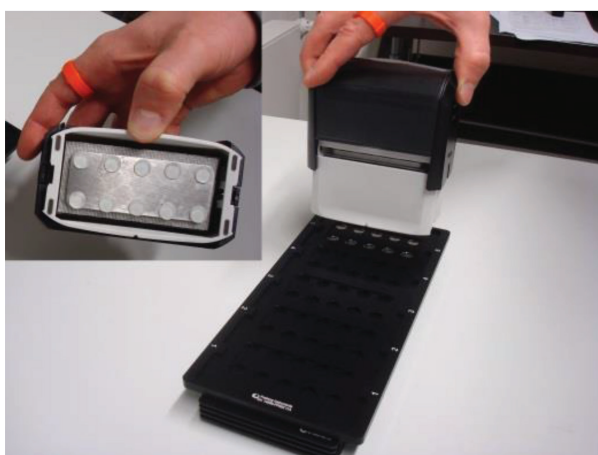
Fig S1. Stamp for simultaneous administration of silicone to ten aliquots for preparation of large (6 mm) aliquots, whereas the stamp for small (e.g. 0.2 mm) aliquots has a different stamp size.
